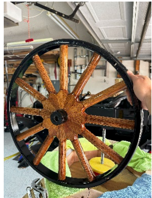
Here is the pressed in spokes prior to drilling holes for the hub bolts.
