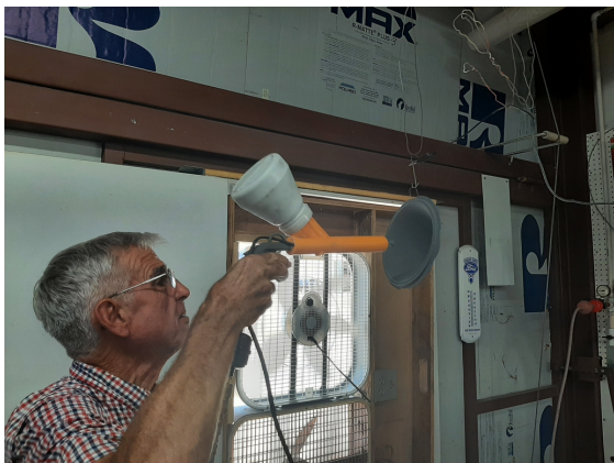
Denny spraying powder on a reflector
