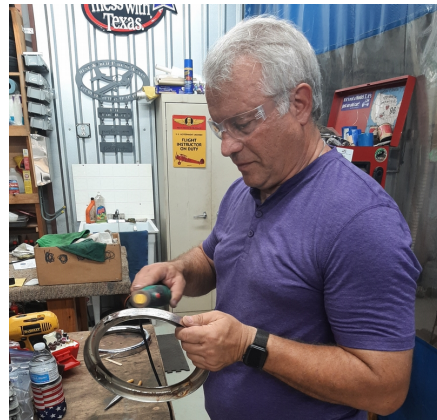
Steve sanding off the salt pits and rust
