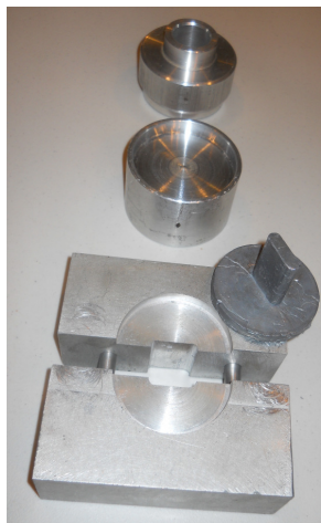
Fixtures designed and made by Frank to cast the lead battery top and roll edges of cylinder
