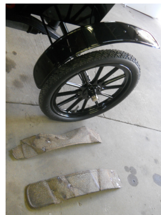
Rear fenders were scratch built. Note the rolled bead.
