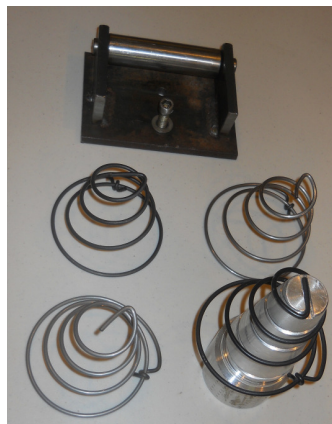
Frank and Benny designed a fixture for winding their own seat springs on a lathe.
