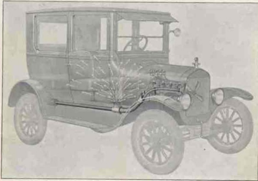
This illustration shows a Kunkel Heater installed and the relative position of the floor register.
