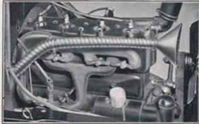
This illustration shows how the intake flexible tube is connected onto the engine and placed back of the fan.
