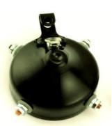
The pacemaker of most Model T engines, in conjunction with the coils and the flywheel magneto, is the timer. It keeps the heartbeat of the ignition sparks appearing when and where they should.
